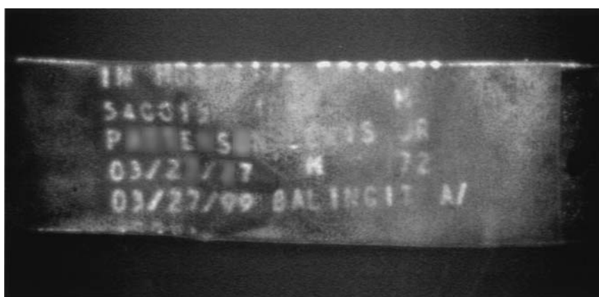
FIG. 6—Infrared luminescence enhancement of the wristband depicted in Fig. 5 revealing all of the original alphanumeric identification information. Portions of which have been intentionally blurred.
